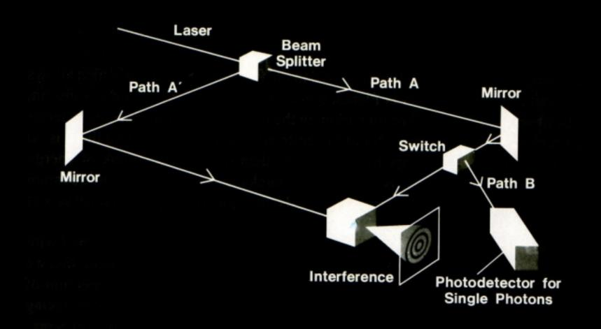
FIGURE 12. A delayed-choice experiment that has been carried out in the laboratory by groups at the University of Maryland and the University of Münich.
